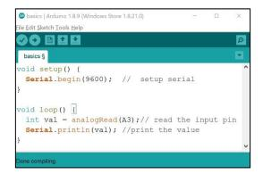
In order to access the serial monitor, we must initialize it first. By doing Serial.begin(9600), we let the Arduino know we are using it now. Technically, the value 9600 can surprisingly be anything! It is just the baud rate of transfer. However, 9600 is the ideal value to use. Sometimes, the serial port will not open when you run the program.
