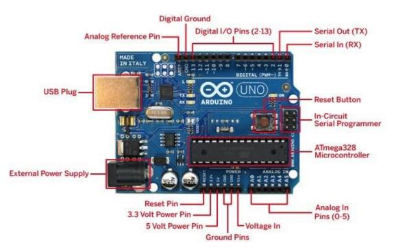
For the majority of projects, only the Digital I/O pins, Analog pins, USB plug, 5-volt Pins, and ground pins will be used. The rest of the pins are used for specialty purposes which will are not required for many projects.
