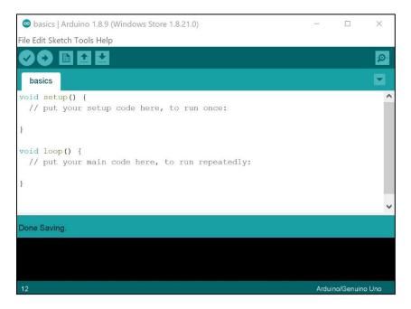
When you open a new file in the Arduino IDE, it should create this framework. If it does not, just enter it in exactly as shown.
